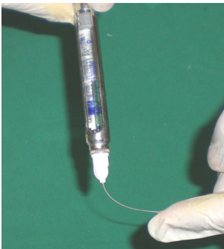
Fig. 2 In vitro assessment of arching of the needle fixed on a syringe
