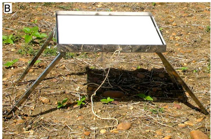
Figure 2. Details of the experimental set. a) 1 × 1 m frame used in the ground-truth field sampling, and b) reference panel for image spectral calibration.
