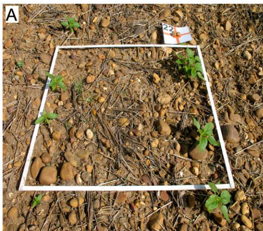
Figure 2. Details of the experimental set. a) 1 × 1 m frame used in the ground-truth field sampling, and b) reference panel for image spectral calibration.
