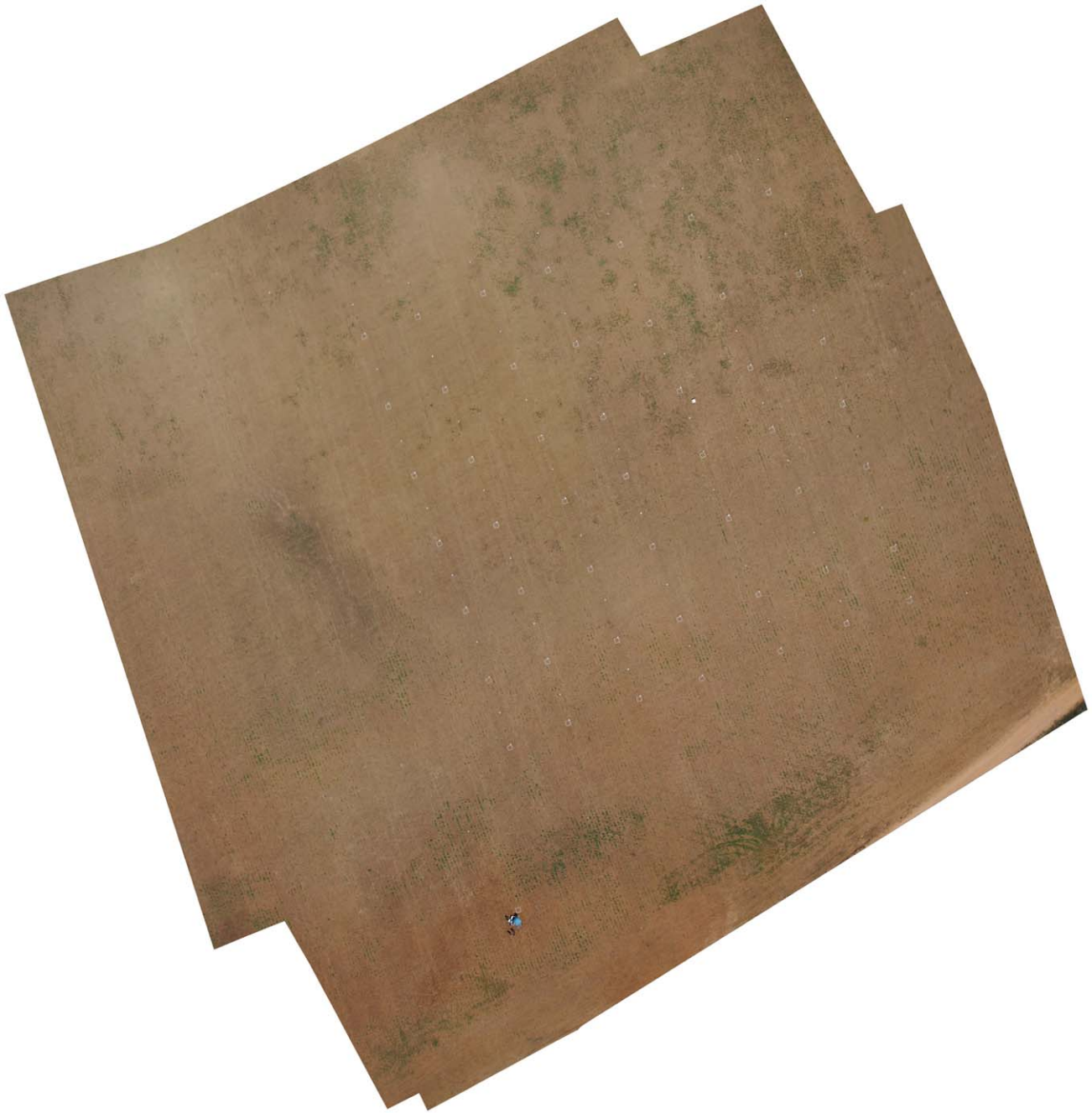
Figure 6. Ortho-mosaic of the whole experimental field. Composed from six individual images taken by the still RGB camera at 100 meters altitude.
