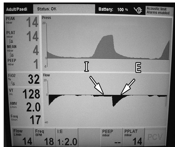
Figure 3: Ventilator display showing the abnormal reverse flow through expiratory unidirectional valve during inspiratory phase (I) and the normal flow during expiration (E)
