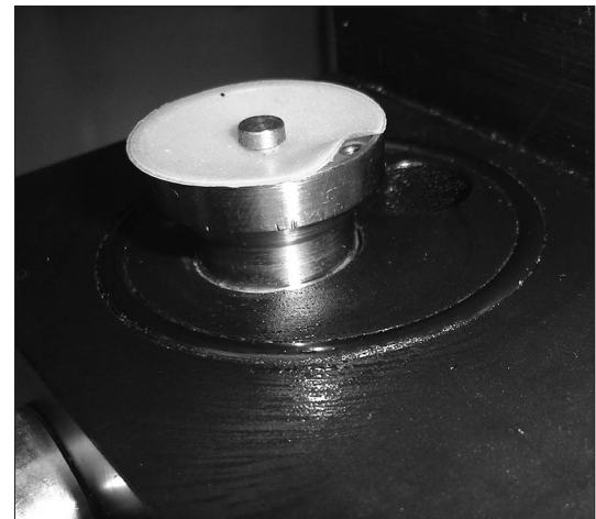
Figure 2: Deformed 'flexible leaflet' of expiratory unidirectional valve (shown after removing the covering dome)
