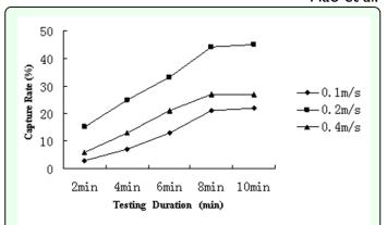
**Figure 5.** Relationship between capture rate and testing duration at three different air-flow speeds (0.1, 0.2, and 0.4 m/s). High quality figures are available online.
