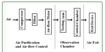
**Figure 2.** A schematic presentation of air-flow and testing. High quality figures are available online.
