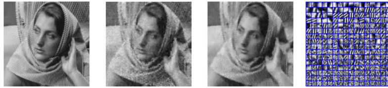
Fig. 5. (From left to right) The original barbara256 image, the noisy and incomplete barbara256 image with the noise standard deviation of 15 and 70% of its pixels missing at random (displayed based upon imputing missing pixels as the average of all observed pixels in a 5 \times 5 neighborhood), the restored image, and the inferred dictionary with its elements ordered in the probability to be used (from top left).
