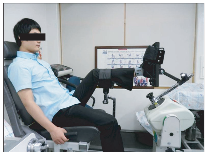
Fig. 1. Isometric strength of ankle dorsiflexor, plantarflexor, everter, and inverter are measured by Biodex System 4 Pro.
