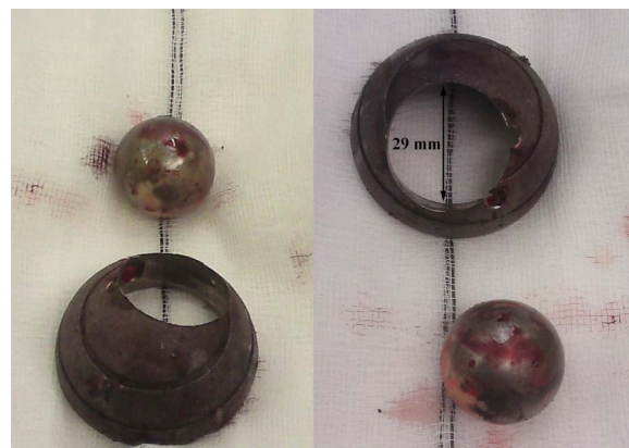
Figure 5 The ceramic femoral head and acetabular shell removed at revision surgery. The femoral head was broken, and the acetabular cup had complete wear.
