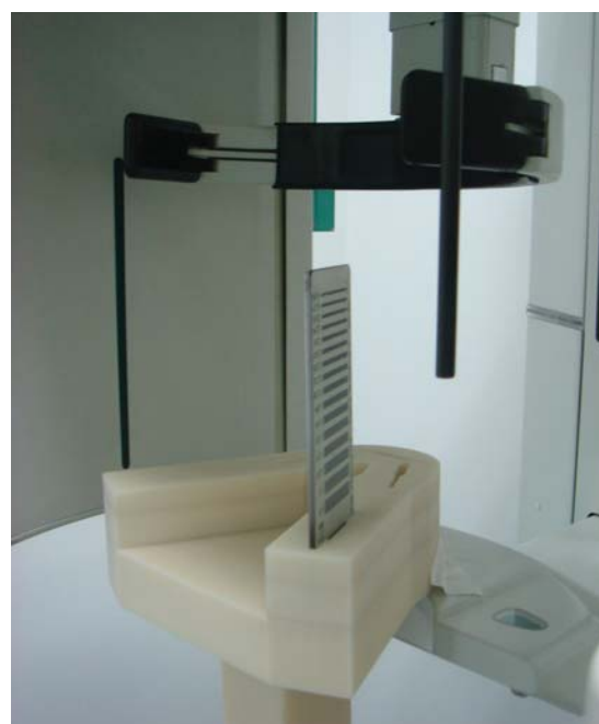
Fig. 5. The selected line-pair phantom is inserted in the right TMJ slit of the phantom stand and these are positioned for panoramic image acquisition.
