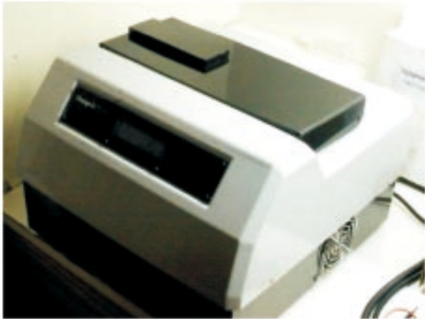
Figure 3. Low cost budget thermocycler Orange G3TB for amplification of M. tuberculosis genome.
