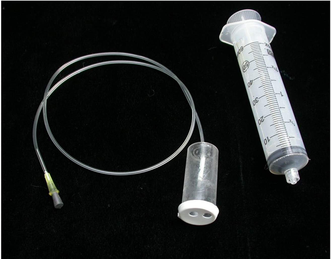
Figure 1. Equipment used to sample soil gas at several depths. The vial was buried openings-down with the fine tubing and syringe needle extending to just above the soil surface. A syringe-full of gas could then be withdrawn from the vial after removing the stopper from the needle. CO 2 in the sample was measure by injecting it into a portable CO 2 analyzer. Four such vials were planted in each borehole at 4 different depths (15, 35, 75, 175 cm).
