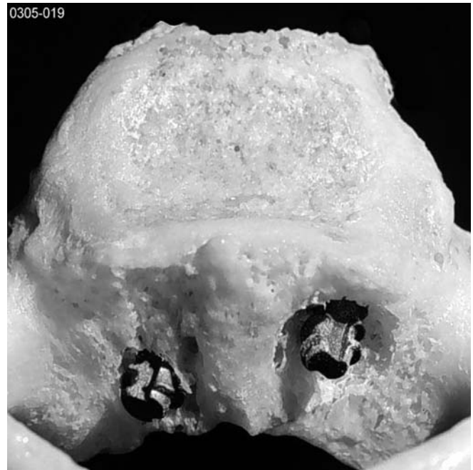
Fig. 1 Photograph of the posterior wall of a cervical vertebra with two screws inserted. A shallow excavation has been performed around the burr hole on the right side to remove the posterior cortical shell, and the cortical shell is intact around the contralateral burr hole
