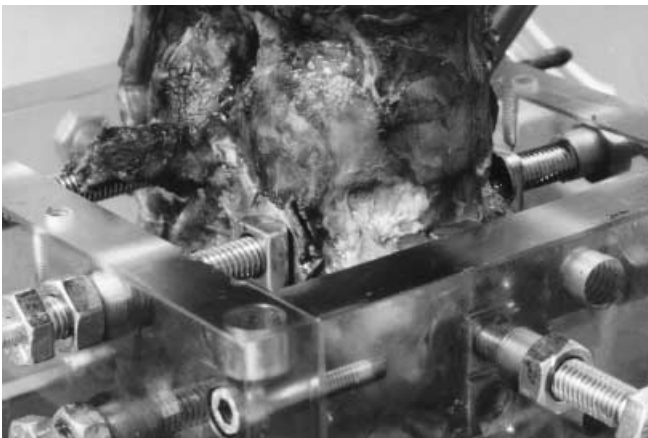
Fig. 1 Fixation of the specimen in the cup in detail
