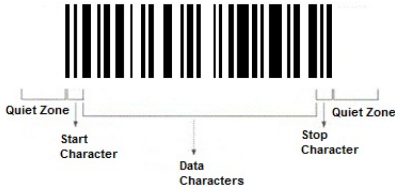
Figure 1. General structure of 1D codes.
