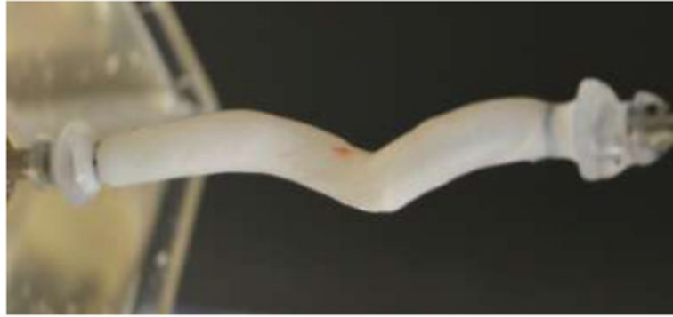
Figure 5. A porcine carotid artery buckled under combined lumen pressure and axial torque. A helical shape is formed.
