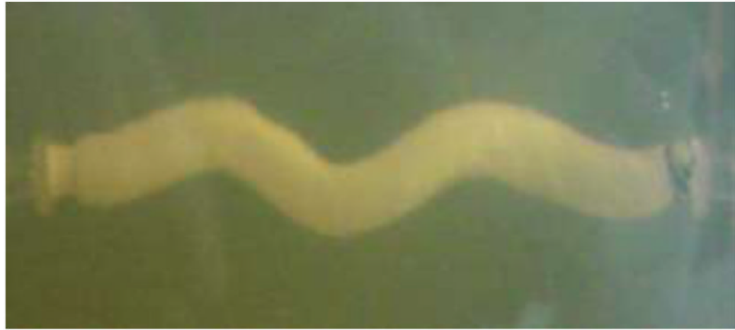
Figure 3. A porcine carotid artery buckled under lumen pressure, within a gelatin matrix simulating surrounding tissue support. A multiple wave tortuous shape is formed.
