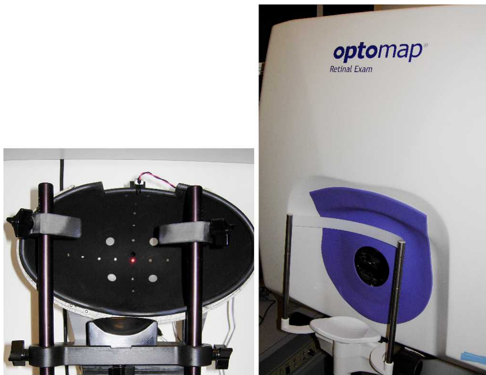
FIGURE 1. Photographs of the bleaching apparatus ( left ) and the Optos P200C SLO ( right ). The two apparatuses sit adjacent to one another in the experimental room, so that the subject can be positioned rapidly in the SLO after a bleaching exposure. The four whitish circular regions in the bleaching apparatus show the locations of the bleaching stimuli; they are glass diffusing plates behind which a cylinder with four LEDs of the same spectral composition can be located precisely. For the subject properly positioned on the chin rest, these diffusing plates subtend a retinal angle of 4.82^\circ at an eccentricity of 15.9^\circ along the diagonal from the red fixation point . Only one of the diffusing targets was used per experiment, and the results reported were all obtained from experiments using the two lower targets, which were imaged on the superior retina.
