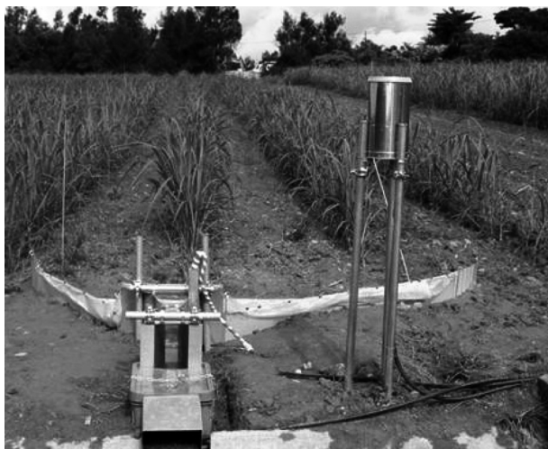
Fig. 5. Parshall flume equipped at the downstream end of sugar-cane field. A rain gage is also placed at the site, as seen in the right hand side of the flume.
