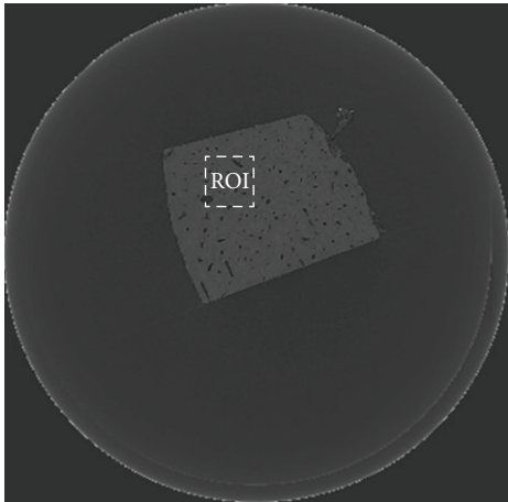
FIGURE 8: The FBP reconstruction of the complete dataset. The image has a large smooth region, so to better demonstrate the details, a region of interest (ROI) is selected.
