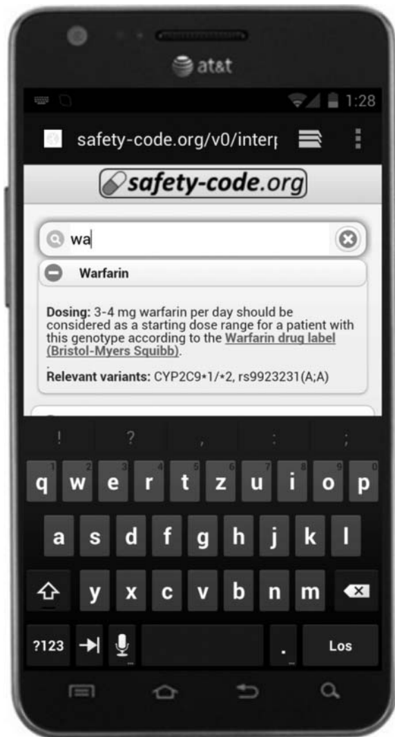
Figure 4 An example of the online clinical decision support algorithms available through the medicine safety code (MSC) server. Through this service, a patient's MSC can be read and interpreted by most common smartphones without requiring the installation of dedicated software.
