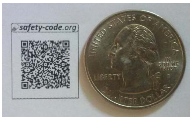
Figure 3 An example of a printed medicine safety code. The quick response code in this example had a side length of 1.15 cm and was readily decoded with the smartphone device used for proof-of-concept testing.
