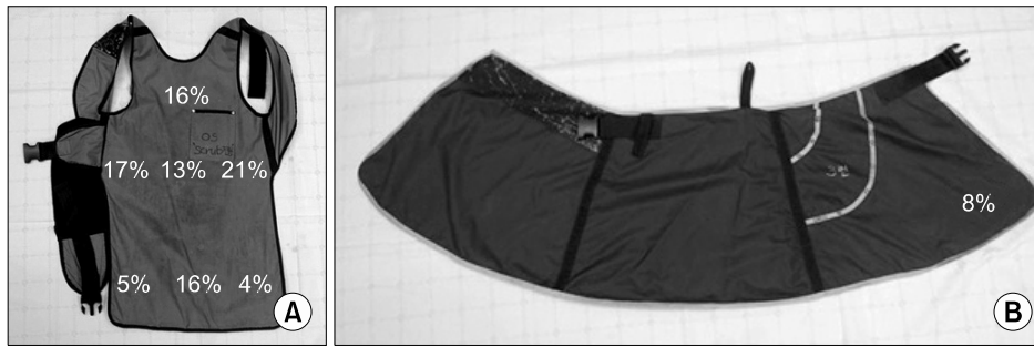
Fig. 2. Damage site and the rate. The most common damaged site of radiation-protective shields was waist of aprons (40%). (A) One-piece type apron. (B) Kilt of two piece type apron.
