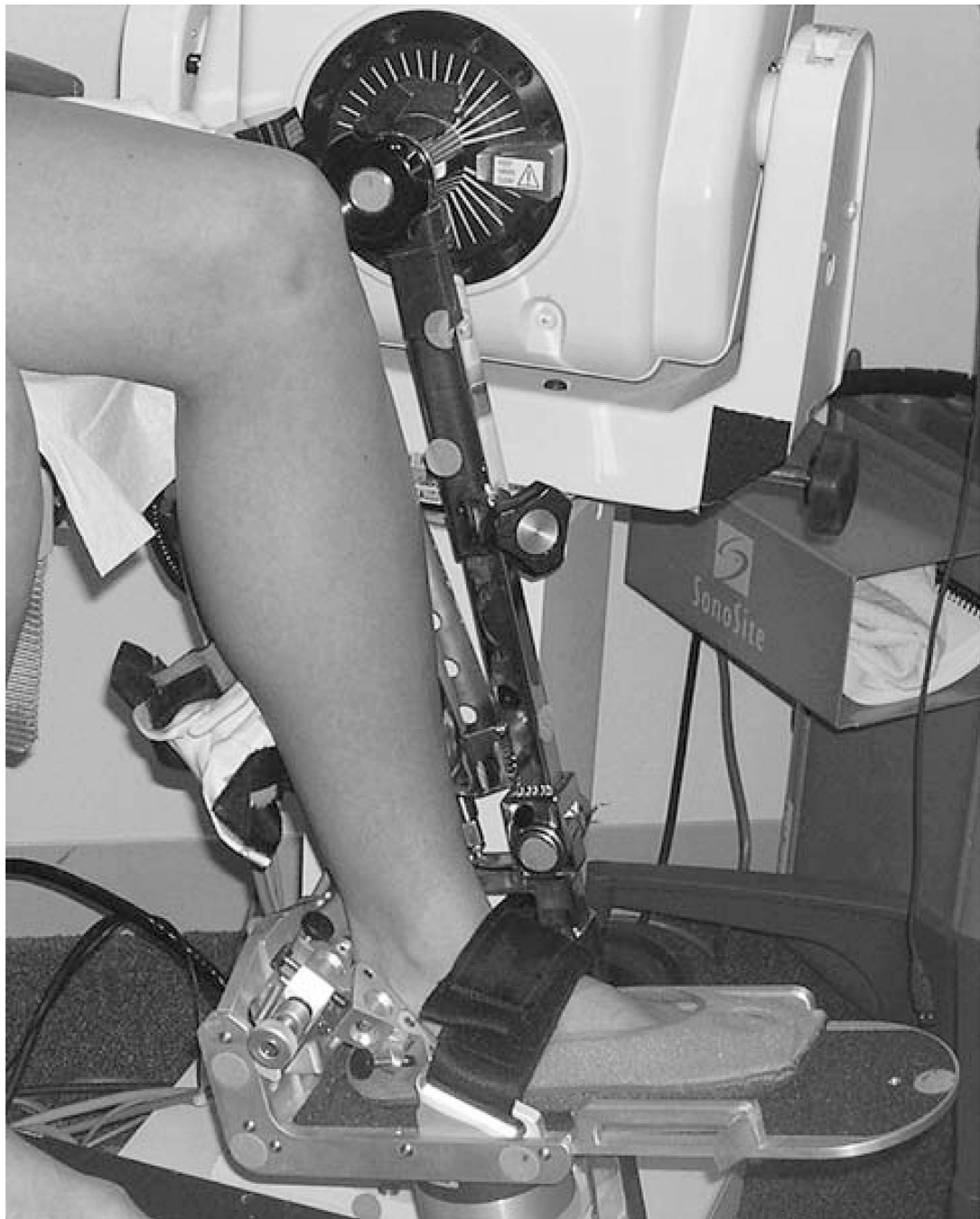
Fig. 1. Apparatus used to move knee and method of foot fixation with ankle at 90°
