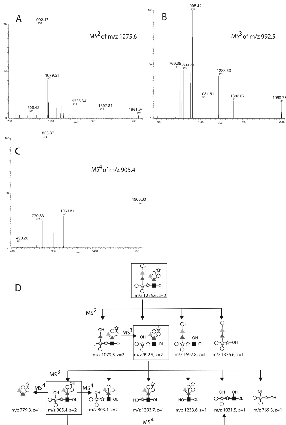
FIGURE 6. ES- MS^n analyses of reduced and permethylated derivatives of the largest glycan released by aq. HF. A , the sample recovered from NMR and reduced with NaBD_4 was permethylated and analyzed by positive ion ES-MS on an Orbitrap instrument. The [M+2Na]^{2+} ion at m/z 1275.6 was isolated and subjected to CID giving rise to the product ion ( MS^2 ) spectrum shown. B , the [M+2Na]^{2+} ion at m/z 992.5 from A was isolated and subjected to CID giving rise to the product ion ( MS^3 ) spectrum shown. C , the [M+2Na]^{2+} ion at m/z 905.4 from B was isolated and subjected to CID giving rise to the product ion ( MS^4 ) spectrum shown. D , the proposed fragmentation pathways corresponding to the ions observed in A – C . Unless otherwise noted, z = 2 ions are [M+2Na]^{2+} and z = 1 ions are [M+Na]^+ . The symbols are as defined in the legend to Fig. 4.
