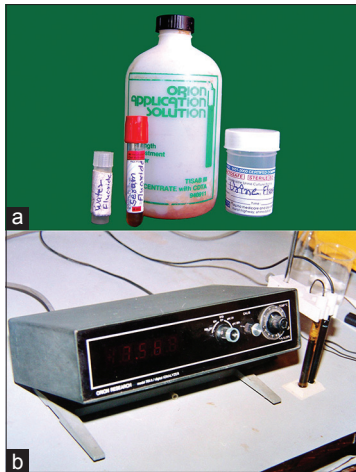
Figure 1: Fluoride estimation by ion selective electrode method
