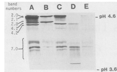
FIG. 1. MUP IEF patterns. Equal volumes of dialyzed urine were loaded onto each lane and focused by the procedure given in Materials and Methods. pH values mark the positions of pI standards (Sigma Chemical Co., St. Louis, Mo.), soybean trypsin inhibitor (pH 4.6), and Aspergillus amyloglucosidase (pH 3.6). Lane A is typical of the pattern observed in males of BALB/cAn, CLA, other Mup-1 a type strains, and intercrossed males which express the MUP-4.1 hi phenotype. Lane B is typical of the pattern observed in females of BALB/cAn, CLA, and others which express the MUP-4.1 hi phenotype. Lane C is typical of the pattern observed in males of BALB/cJPt family 1 and other males which express the MUP-4.1 lo phenotype. Lane D is the pattern observed in males of BALB/cJPt family 2 and other males which express the MUP-null phenotype. Lane E is the pattern typical of BALB/cJPt family 1 and family 2 females and intercrossed females that express the BALB/cJ phenotype.
