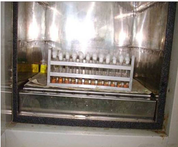
Fig. 3 Incubation of test tubes carrying the test specimens inoculated with test microorganisms
