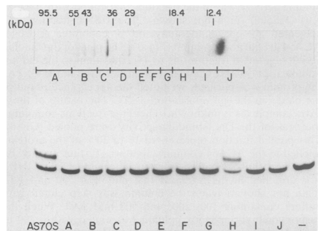
FIG. 5. Identification of the proteins in the crude extract that contains NTS-binding activity. Proteins from the AS70S fraction were fractionated on an SDS-containing 15% polyacrylamide gel. The gel was then sliced into several regions, designated A through J, as shown at the top of the figure. Proteins from each gel slice were eluted, renatured as described by Hager and Burgess (18), and analyzed for their specific DNA-binding activity (bottom panel). Only proteins that eluted from gel slice H contained the same activity as p16.
