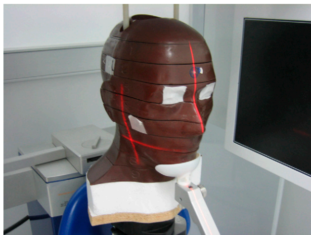
Figure 1 Phantom positioning using the KaVo 3D eXam’s light localizer (KaVo Dental, Biberach, Germany)
