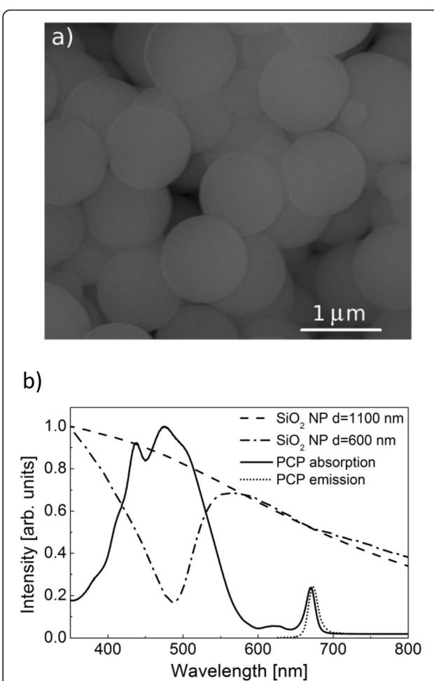
**Figure 1** Scanning electron microscopy image and optical spectra of the silica nanoparticles. (a) Scanning electron microscopy image of the silica nanoparticles with a diameter of 1,100 nm. (b) Optical spectra of silica nanoparticles with diameters of 600 nm (dash-dot) and 1,100 nm (dash) compared to absorption spectrum of the PCP complex solution (solid) as well as its fluorescence (dot).
