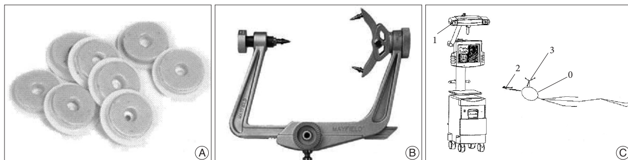
Fig. 1. A : Fiducial markers. B : Mayfield frame as pinning fixation system. C : The setting of classical optical neuronavigation (0 : patient's head, 1 : infra-red camera, 2 : navigation pointer, 3 : reference frame).
