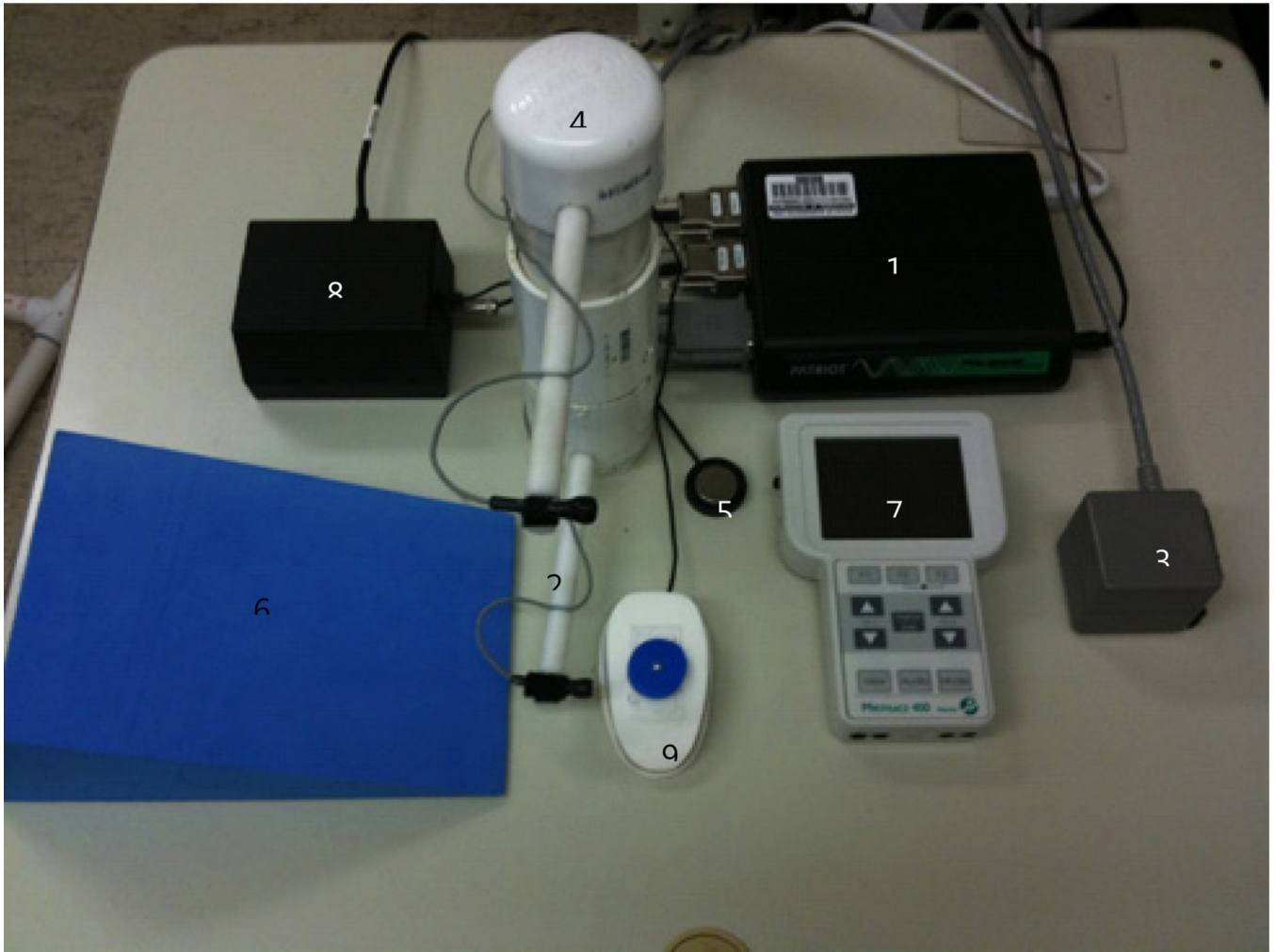
Figure 1. System Components: 1. The Patriot™ tracker, 2. Sensors, 3. Transmitter, 4. Spring calibration plunger, 5. Foot switch controller, 6. Hard foam wedge for scapular support and positioning, 7. Surface EMG unit for muscular activation level feedback, 8. USB Analog to digital converter, 9. Early prototype hand force transducer. Laptop computer not shown.
