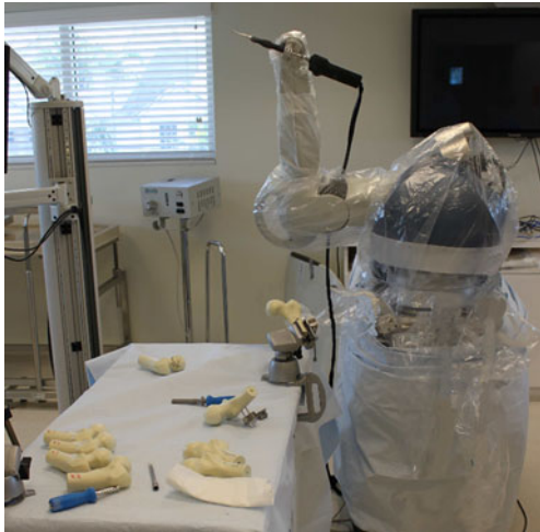
Fig. 5. Photograph of the MAKO robotic arm being used to perform femoral osteochondroplasty in sawbone models.
