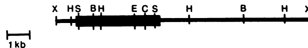
FIG. 1. Restriction enzyme maps of (a) the enhancer-deleted variant of the pZipNeoSV(x)1 retrovector and (b through e) the retrovector-containing Xba I fragments isolated from the parental EN/NIH 2-4 and 2-20 cell lines by a previously described protocol (43). Each cell line contains two integrants of the enhancer-deleted retrovector. Thin and thick lines represent cellular and retrovector DNA, respectively. enh, enhancer; ori, origin of replication. Restriction enzymes: X, Xba I; S, Sac I; C, Clal ; E, Eco RI; B, Bam HI; H, Hind III; Bg, Bgl II; N, Nde I.
