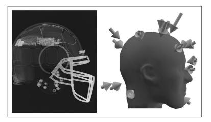
**Figure 1.**X-ray image showing the HIT System encoder located along the crown of a Riddell helmet. Arrows around the red headform indicate individual impacts with tail length suggesting magnitude. 40 ms of data are recorded as representative of the impact: 12 ms prior to impact and the 28 ms following. HIT, Head Impact Telemetry.
