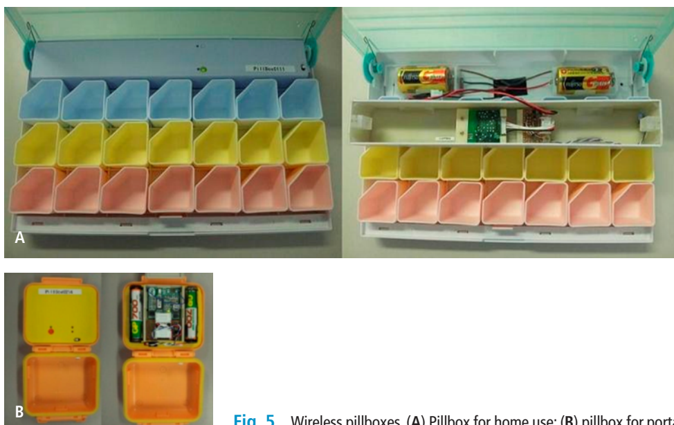
Fig. 5 Wireless pillboxes. (A) Pillbox for home use; (B) pillbox for portable use.
