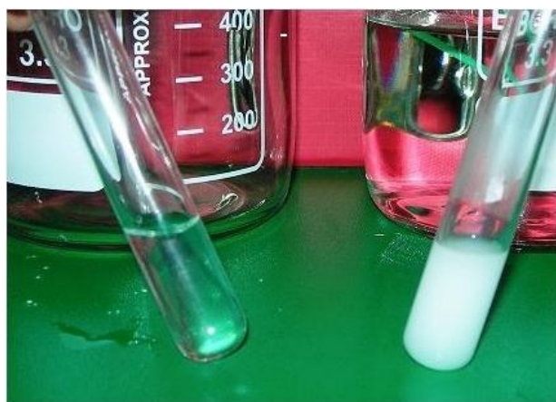
Fig. 13. Visual observation of macroscopic phase separation of aqueous solution of cross-linked P (NIPAAm-MAA-HEM)-1 hydrogel.
