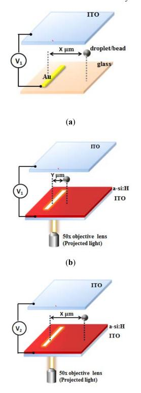
**Figure 4.** The repelled distance generated by the DEP electrode and the ODEP virtual electrode for a 20  $\mu$ m droplet. The VTR is calculated as 1/3 in this case when comparing the repelling distance generated by DEP and ODEP forces.
