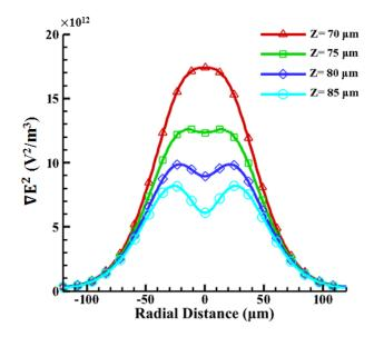
**Figure 8.** A comparison between the experiment results and simulation data. The emulsion droplet has an applied voltage of 60 Vpp with a driving frequency of 100 kHz in the 100  $\mu$ m spacer.
