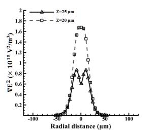
**Figure 11.** Comparison between experiment results and simulation calculations for polystyrene beads at an applied voltage of 36 Vpp (12 Vpp for the transformed voltage) with a driving frequency of 100 kHz and a 100  $\mu$ m spacer.
