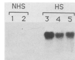
FIG. 4. Camptothecin partially inhibits transcription of hsp28 . The level of hsp28 RNA was measured from an RNA blot. Cells were treated in the following ways. Lanes 1, RNA from noninduced cells treated with 0.2% dimethyl sulfoxide; 2, RNA from noninduced cells treated with 10 \mu M camptothecin for 40 min; 3, RNA from cells heat shocked for 40 min; 4, RNA from cells treated for 5 min with 10 \mu M camptothecin at room temperature followed by a 40-min heat shock; 5, RNA from cells heat shocked for 5 min and then treated with 10 \mu M camptothecin for 35 min at 36°C. The ethidium bromide-stained gel indicated that each lane contained comparable amounts of total RNA. The RNA blot was analyzed by using the Hind III- Pst I fragment from 88.1 (9) which hybridizes to hsp28 and approximately 400 base pairs flanking each side of the gene.
