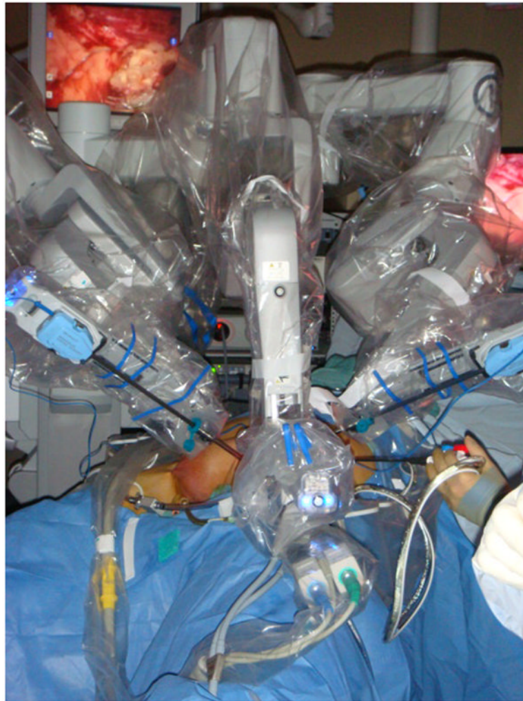
FIG. 2. Docking alignment for the RAVEIL procedure. The machine is docked at about a 45° angle from the opposite side of the leg being operated on.
