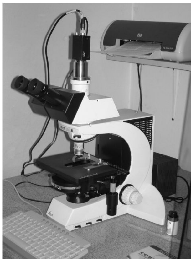
Figure 1. An upright Leica microscope used for tethered particle motion experiments. The small CCD camera is mounted on a 1X coupler attached to the trinocular.
