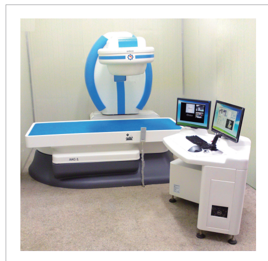
Figure 2. The front view of the magnetic-controlled capsule system.
