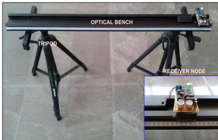
Figure 11. Test bench used to position the receiver node in different positions.
