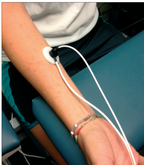
Figure 1. The Moor laser flow meter with the surrounding thermode to heat the skin.
