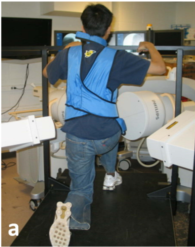
Figure 1. (a) Subject performing a quasi-static single-legged lunge (right knee) in the DFIS. (b) Reproduction of the kinematics of the knee in a virtual DFIS. (c) Knee position at high flexion of one subject recreated in the virtual environment.
