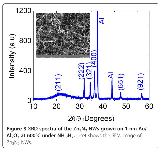
**Figure 3** XRD spectra of the  $\text{Zn}_3\text{N}_2$  NWs grown on 1 nm Au/ $\text{Al}_2\text{O}_3$  at  $600^\circ\text{C}$  under  $\text{NH}_3:\text{H}_2$ . Inset shows the SEM image of  $\text{Zn}_3\text{N}_2$  NWs.
