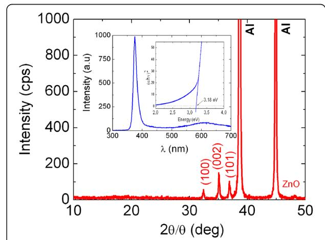
**Figure 2** XRD spectra of  $\text{ZnO}$  NWs' lower trace. Inset shows the PL of the  $\text{ZnO}$  NWs and square of the absorption versus energy.
