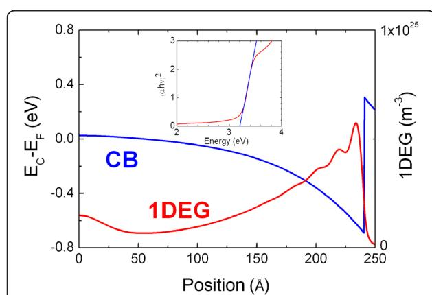
**Figure 4** Self-consistent conduction-band edge potential with respect to the Fermi level.  $E_C - E_F$  ( $E_F = 0$  eV) versus radial position for a 50-nm diameter  $\text{Zn}_3\text{N}_2/\text{ZnO}$  core-shell NW. The core has a radius of 24 nm. Inset shows the absorption squared versus energy for the  $\text{Zn}_3\text{N}_2$  NWs grown on 1 nm Au/ $\text{Al}_2\text{O}_3$ .
