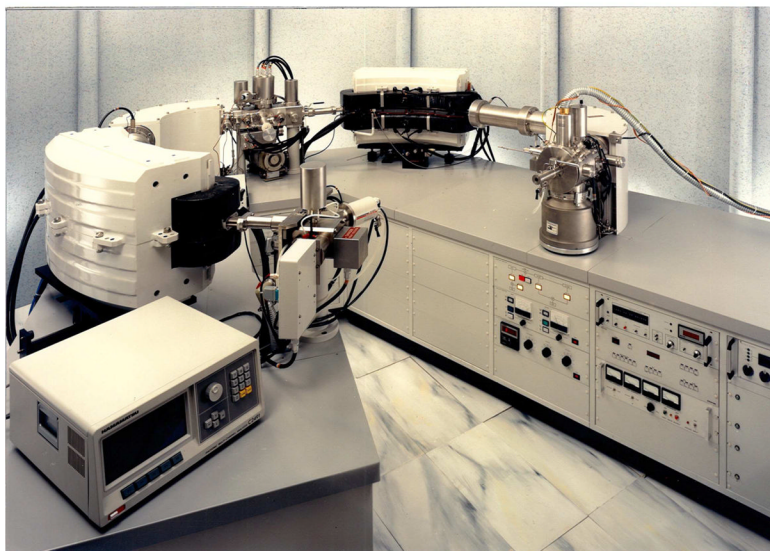
Figure 3. Kratos four sector ( EBEB ) mass spectrometer with fast atom bombardment (FAB) ion source. (Photo courtesy of Andrew Bowdler, Kratos Analytical Instruments).
