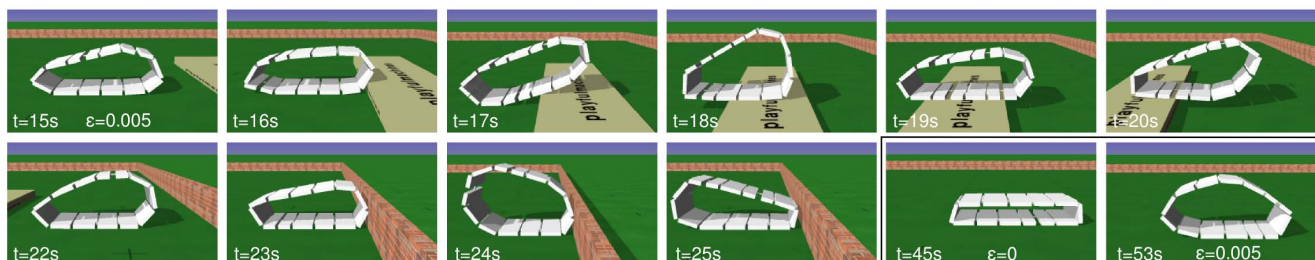
Figure 8. Armband robot surmounting an obstacle and inverting speed at a wall. Screen shots from the simulation for Fig. 7. The order is row-wise from left to right. The last two pictures show the situation after switching off the parameter dynamics \varepsilon = 0 for a few seconds (the robots stops) and enabling it again (starts moving). doi:10.1371/journal.pone.0063400.g008
