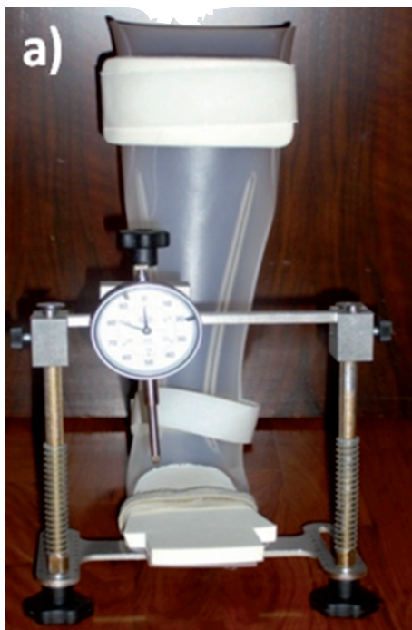
Figure 2. a) Modified Klaue device used in this study. b) The foot is placed in the orthosis at 90° to the leg, ankle in neutral position and it is immobilized in three points: calf, ankle, and midfoot.
