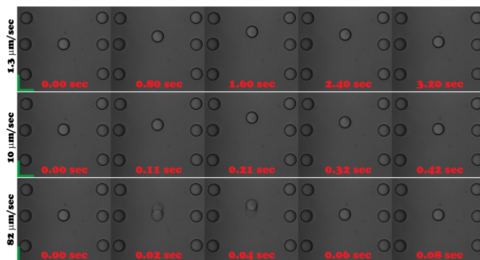
Figure 3. Two rows of traps are made using 6 operator defined and controlled holographic traps. An additional conventional trap is defined between the two rows and its position is adjusted at various speeds as indicated. The bead is moved to a maximal spatial displacement of 4.1 \mu\text{m} and then back to the original location. A video of bead motion is recorded at 47 fps. As trap repositioning speed is increased, progressively larger motion blur is observed in the video. The objects trapped are refractive beads (see Table of Materials for more details) suspended in de-ionized water. Frame timings are shown in red. Trap repositioning speed is shown for each row. Green scale bars correspond to 5 \mu\text{m} in each direction.
