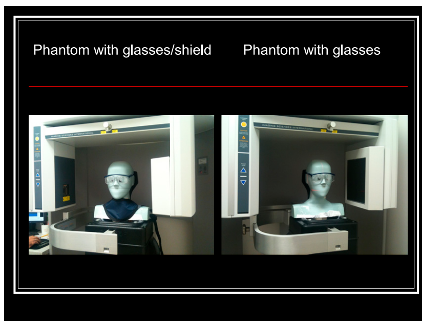
Figure 1 Phantom with glasses and thyroid shield and glasses and no thyroid shield
