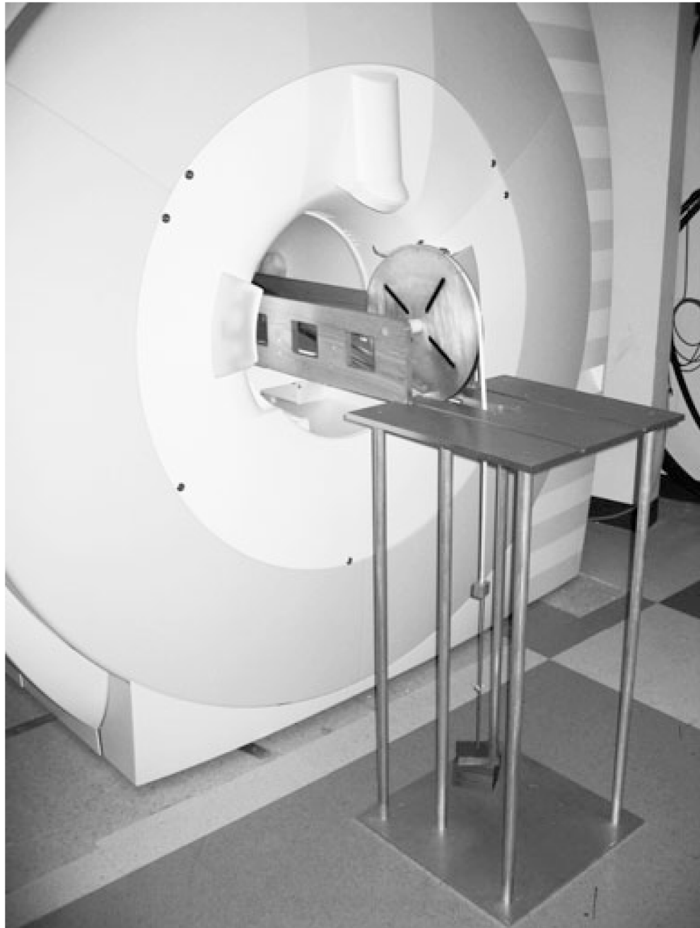
Fig. 2. Photograph of distal portion of MR-compatible exercise device inside the magnet bore, supported by the weight stand assembly
