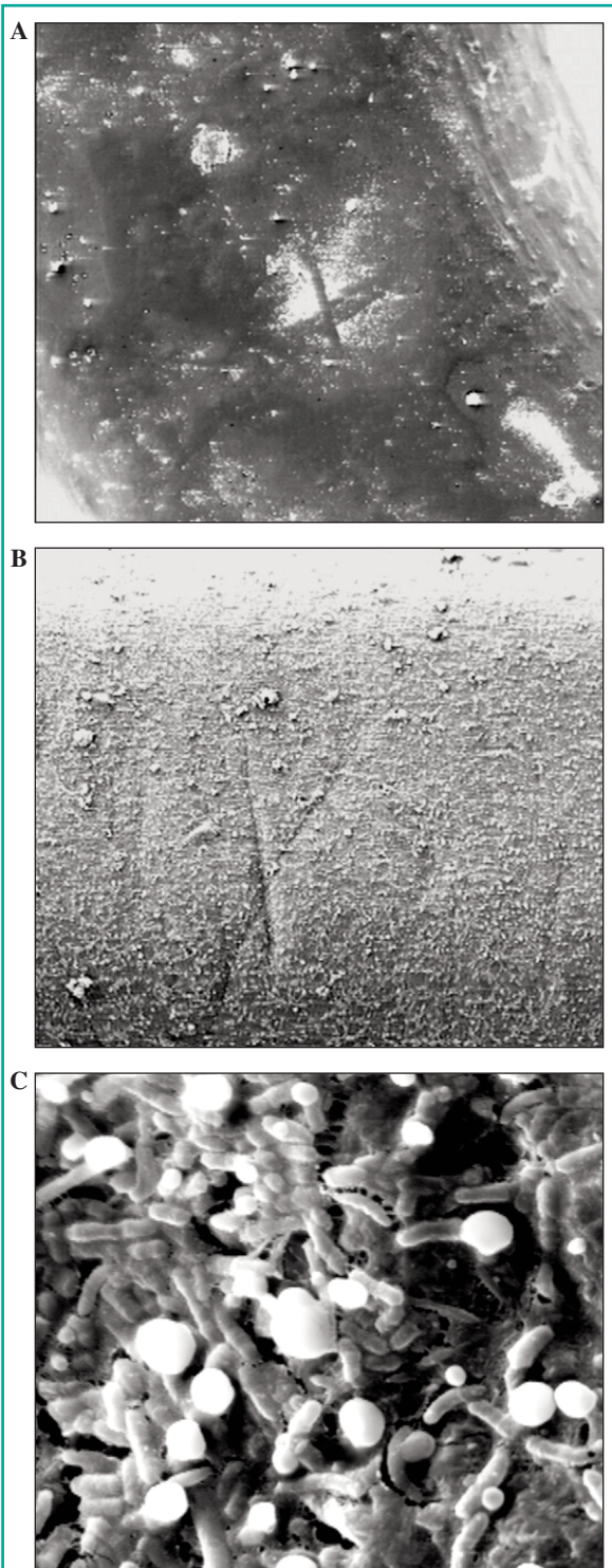
Figure 3 SEM micrograph of grey, polyurethane, ring-shape ligatures (GR). Before use (A-x200) and after 4 weeks of permanence in oral cavity at original magnification x200(B) and x5000(C).
